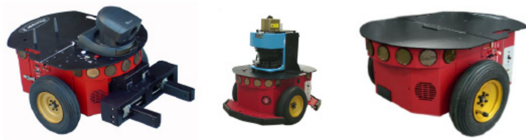
Figura 4.1. Pioneer DX2 de Active Media Robotics
