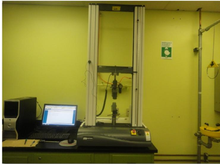
Figura 2.12 Máquina Universal INSTRON 3365
