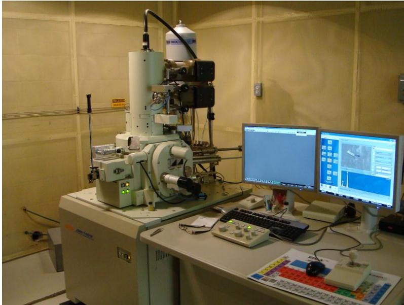
**Figura 2.8** JSM-4701 F Scanning Microscope
